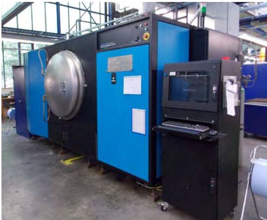
Abbildung 7: MIM Sinterofen (Elnik Systems).
